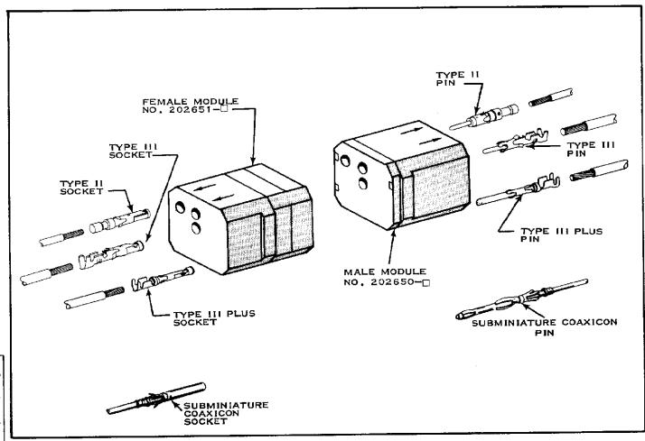
1. These instructions cover the Series "G" Modules shown in the illustration and selection and crimping of Contacts for use in the Modules. These Modules are used in A-MP Series "G" Connectors. To assemble Modules in Connectors refer to AMP Instruction Sheet No. 7184 which is packaged with the Connectors.
