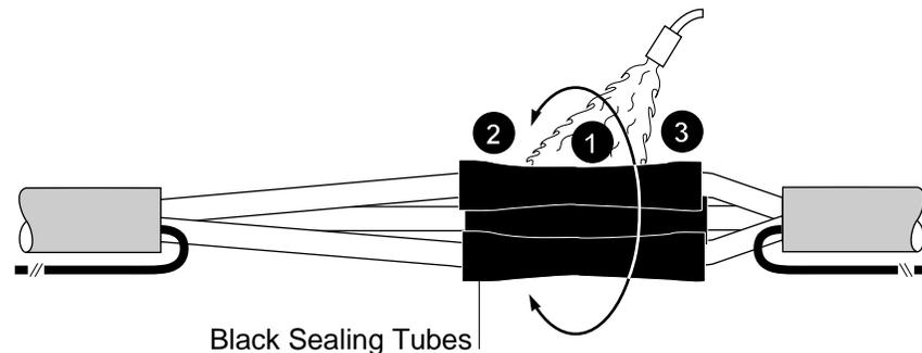
**Note:** Do not point the flame directly at the cable insulation.
