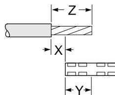
$$\text{"Z" Insulation Cutback} = \text{"X" Expansion Gap} + \text{"Y" 1/2 Length of Connector}$$
