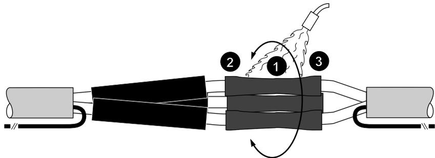
**Note:** Do not point the flame directly at the cable insulation.
