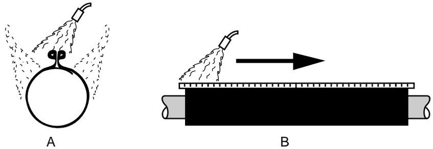
Begin shrinking at the center of the sleeve and work toward each end. Apply heat until the sleeve is fully shrunk and the heat-sensitive green paint is completely converted to black. Continue heating the rail/channel area for another 5 seconds per foot. A white line should be visible in the channel gaps indicating sufficient heating.
