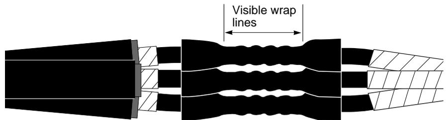
Post heat the connector area until the tube surface is smooth and the underlying SRM wraps are no longer visible.
