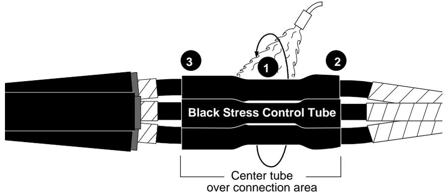
The rings from the SRM wraps may be visible as the tubing shrinks.
