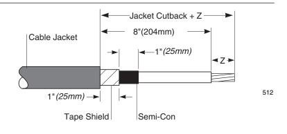
Remove the backing from a piece of copper foil provided and tape over the end of the shield as shown.
