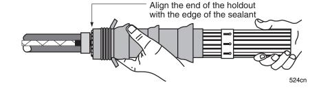
Slide the termination off the holdout with a twisting motion holding the termination that is on the holdout in one hand and pulling the holdout with the other.
