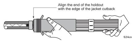
Twist clockwise and counterclockwise while pulling out
