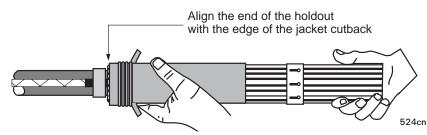
Twist clockwise and counterclockwise while pulling out
