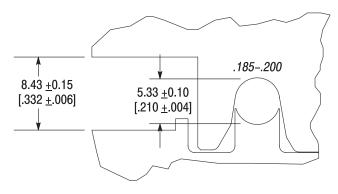
For 5.08-5.46 mm [.200-.215 in.] Insulation Dia.
