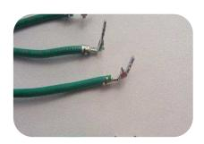
5. Inspect all contacts for straightness and damage. Confirm compliance with 114-106118 for PTL wire-to-wire contacts or 114-106147 for PTL MFBL contacts. Do not attempt to straighten bent or distorted contacts. If any contact does not comply or is questionable, cut it from the wire directly behind the stabilizer, re-strip the wire, and crimp with a new contact. The new contact must have the same part number as the one removed. Refer to the 114-document for crimp requirements.
