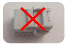
Discard the housing as it may have internal damage. It is important that the housing **not** be re-used because internal damage cannot always be easily determined.
