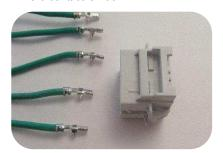
Insert all contacts into a new housing. There will be a slight audible click when the contact latches onto the housing.
