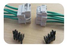
1. Remove the TPA from the back of the housing and discard it.
