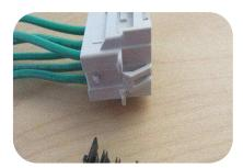
Give a slight tug to all wires to ensure that the contacts are latched onto the housing.
