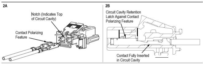
c. Gently pull the wire to ensure that the contact is locked in place. See Figure 2, Detail B.
