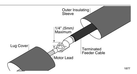
**Note:** MCK insulating caps are designed to accommodate the largest lugs normally used. However, many installations require shorter caps due to space limitations. MCK can be trimmed to any desired length as long as the following rules are observed.
