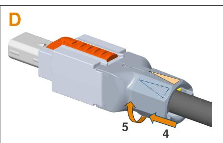
Afterwards while moving the nut in direction (4) the triangle on the outer surface of the nut must initially located on the left side of the gap between the half shells. This closes the strain relief and contacts the cable shield. Finally turn (5) the bayonet nut clock-wise against the stop position as shown.
