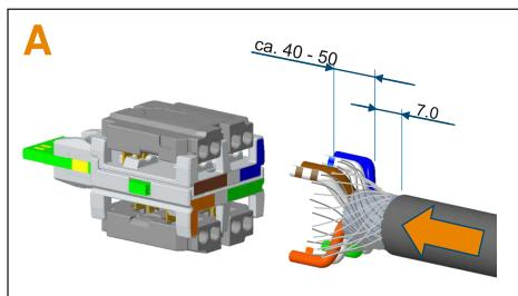
First put the nut on the cable. Remove the insulation of the cable preferably with a professional stripping tool according to the above dimensions. Then pass the wires through the openings matching the color code. The shielding braid must be moved along the eight wires until their individual insertion positions at the holes of the housing to ensure the optimum position for the subsequent shielding connection.
