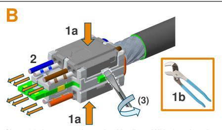
Close (1) the connection unit with pliers. With that the wires are automatically cut and terminated. Remove (2) the protruding ends of the wires.
