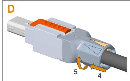
Afterwards while moving the nut in direction (4) the triangle on the outer surface of the nut must initially located on the left side of the gap between the half shells. This closes the strain relief and contacts the cable shield. **Finally** turn (5) the bayonet nut clock-wise against the stop position as shown.
