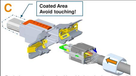
Push the connection unit with cable into the housing until it is flush with its rear surface. If the orientation is correctly selected, the connection unit can be easily inserted, otherwise it should be reoriented by half a turn. Now close the two movable wings manually. Press the two swiveling half shells against each other with force so that the bayonet nut can catch all four of its pointed ends.
