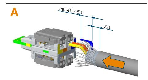
First put the nut on the cable. Remove the insulation of the cable preferably with a professional stripping tool according to the above dimensions. Then pass the wires through the openings matching the color code. The shielding braid must be moved along the four wires until their individual insertion positions at the holes of the housing to ensure the optimum position for the subsequent shielding connection.
