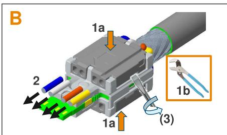
Close (1) the connection unit with pliers. With that the wires are automatically cut and terminated. Remove (2) the protruding ends of the wires.
