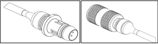
Figure 7 Completed NettWarrior Plug and Receptacle Assemblies with Braid Terminated using Band Strap.
