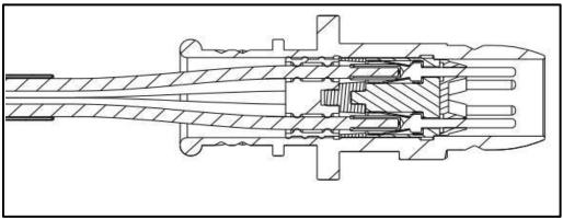
Figure 5 - Cross Section of Plug Connector with Pins Installed
