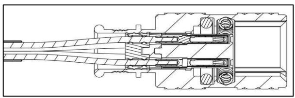
Figure 6- Cross Section of Receptacle Connector with Sockets Installed
