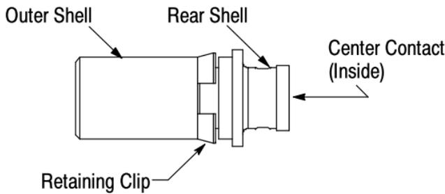
Figure 1: SMPM Panel Mount Cable Plug
