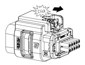
Hold the housings, and if applicable, simultaneously press the optional CPA, then pull the plug assembly and mating connector apart. DO NOT pull the wire bundle.
