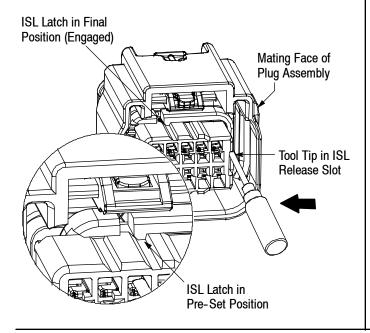
2 Insert the tip of the tool under the internal latch beam of the contact cavity of the contact to be removed.
