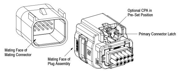
1 Holding the housings, align the mating face of the plug assembly with the mating face of the mating connector, and push them together.
