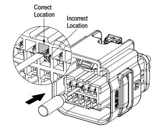
**3** Rotate the tool handle toward the opposite row of contact cavities until the internal latch beam releases the contact locking latch and, simultaneously, pull the wire until the contact is out of the plug assembly.
