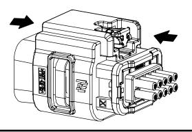
**2** Push the CPA inward until there is an audible click (the primary connector latch should be engaged). The CPA is now in the locked position.
