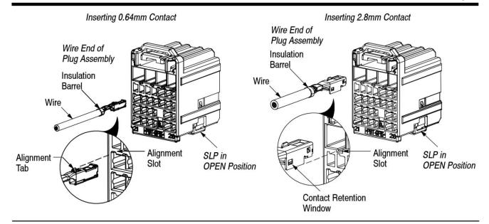
5. After all contacts are inserted, push the SLP into the housing until it in the CLOSED position. The SLP is in the CLOSED position when it is flush with the housing and the two latches engage the housing. Check to make sure that the entire SLP is seated against the housing, and that there is no gap between each latch and the housing. See Figure 3.
