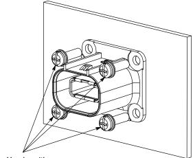
Secure Header with Four M4 Fasteners
