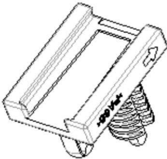
Figure 42 Insert the fuse box housing on the plastic clip as shown in Fig. 42. The clip is fixed on the vehicle body. An audible click sound is to ensure the proper mounting clip.
