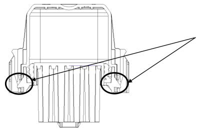
Cover Locking with Fuse Box housing. Both snaps are locked.
