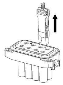
Pull the fuse puller in the upward direction to disengage the fuse from the terminals as shown in Figure 11.
