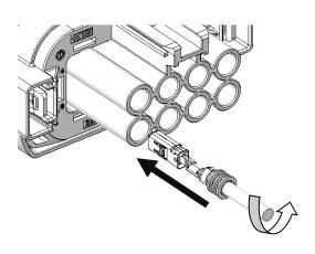
Orient the terminal as shown in figure 5 and insert it in the housing cavity. The terminal locks with a click sound.
