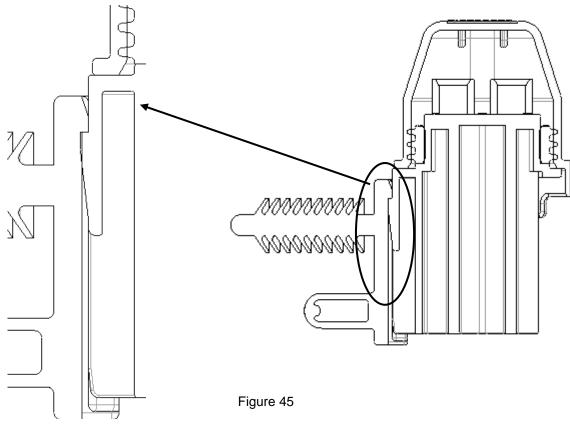
Figure 45 shows the engaged position of mounting clip to the raised bump in the housing.
