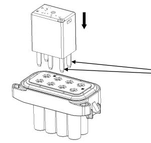
Orient the Relay as shown in Figure 7 and push the Relay in the shown direction.
