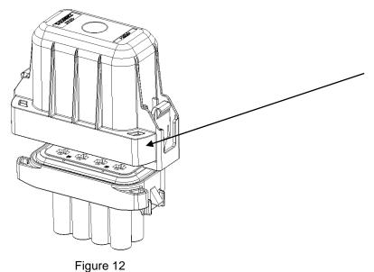
Poka-Yoke designed on cover will not allow the insertion of the cover in reverse direction. See Figure 12.
