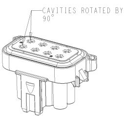
Figure 1 2319023-1 8P Mini Fuse Housing Assembly
