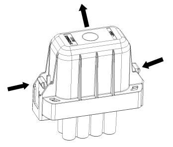
Press both the cover snap locks simultaneously as shown in figure 16 and pull the cover in the upward direction to release it completely.
