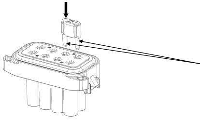
Orient the Fuse as shown in Figure 6 and push the Fuse in the shown direction.
