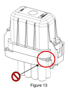
Figure 13 shows wrong orientation of cover during assembly.
