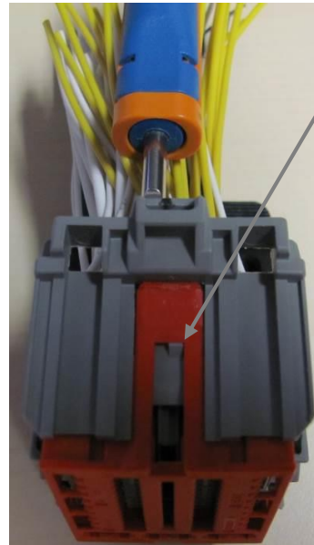
Figure 8: Insert TE extraction tool TE PN 0-1452426-1
