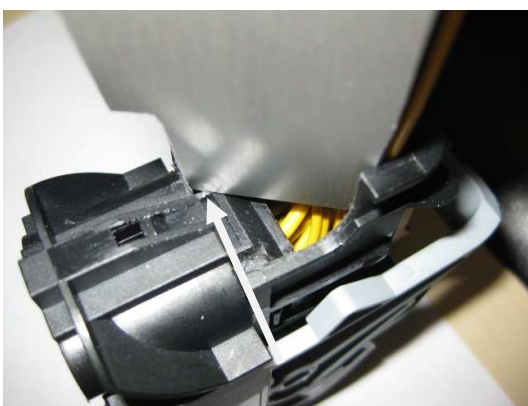
Figure 10: 38 posn, mixed, receptacle housing, radial seal Contact extraction, cap removal
