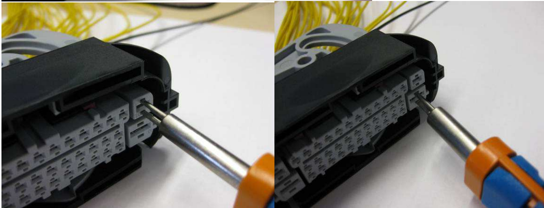
Figure 13: 38 posn, mixed, receptacle housing, radial seal Contact extraction
