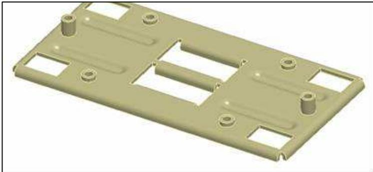
Fig 5a. Recommended back plate design (Based on AMD design)
