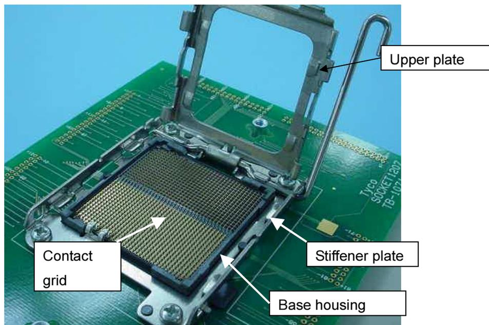
Fig.3. : Socket in "Open" position
