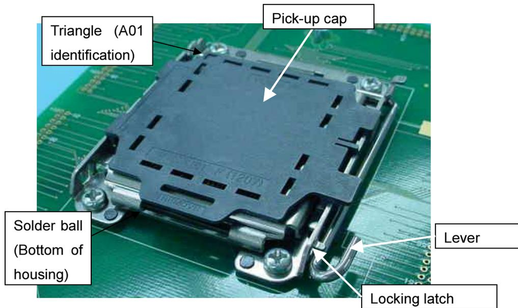
Fig.2 : Socket in "Close" position
