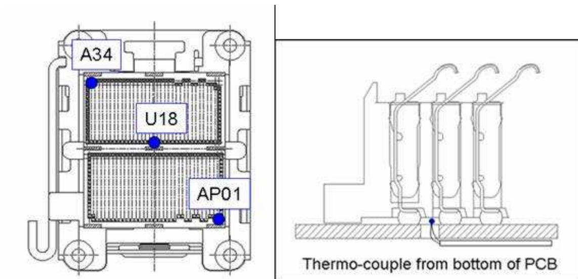
Fig 9) Recommended temperature measurement position for SMT
