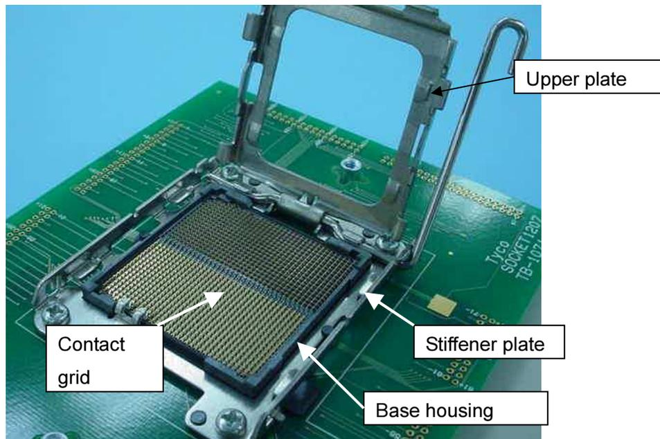
Fig.3. : Socket in "Open" position
