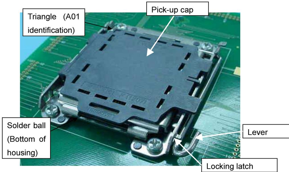
Fig.2 : Socket in "Close" position
