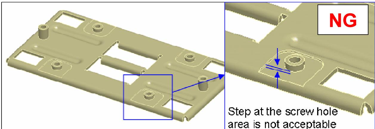
Fig 5b. NOT acceptable back plate design (it has step at screw hole area)
