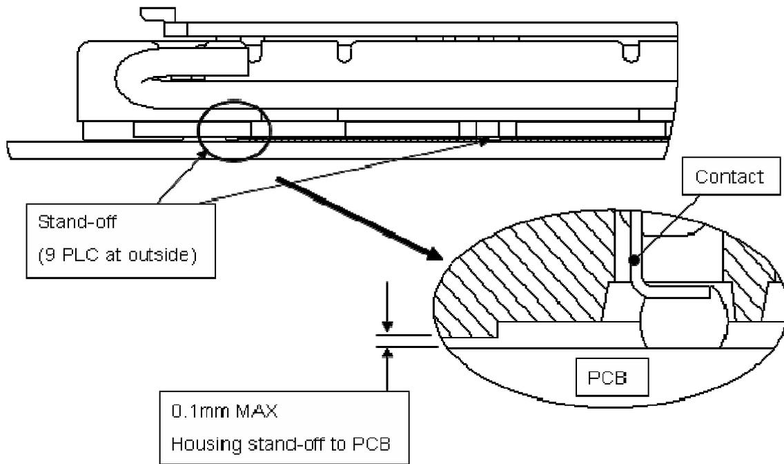
Figure 10). After SMT on PCB
