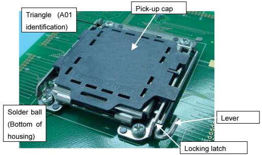
Fig.2: Socket in "Close" position
