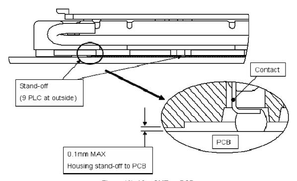
Figure 10). After SMT on PCB
