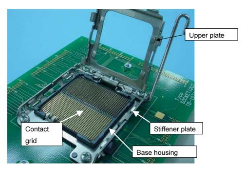
Fig.3.: Socket in "Open" position
