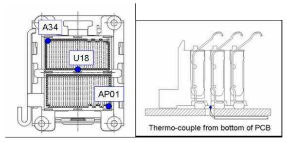
Fig 9) Recommended temperature measurement position for SMT
