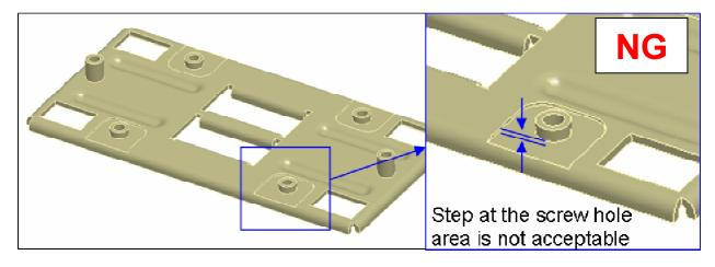
Fig 5b. NOT acceptable back plate design (it has step at screw hole area)
