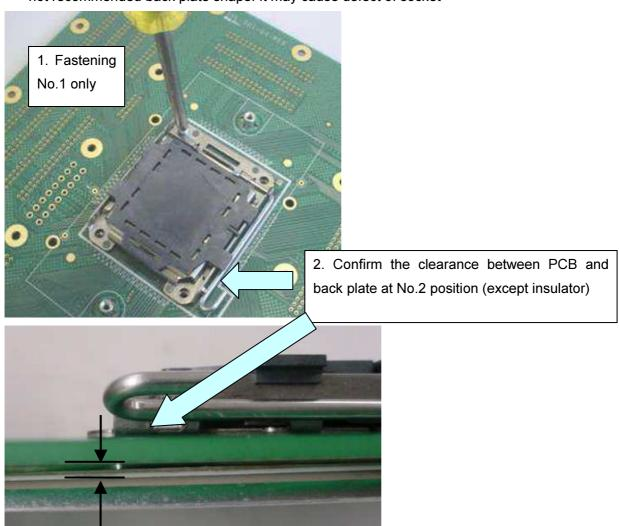
Fig 7 Confirmation of clearance between PCB and back plate
