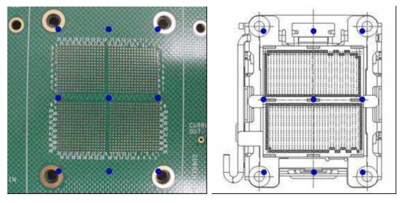
Fig.4 Recommended measurement position of PCB warpage after SMT
