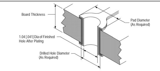
NOTE: Board thickness shall be 2.36 mm [.093 in.] for standard connectors or 1.57 mm [.062 in.] for connectors with boardlocks.
