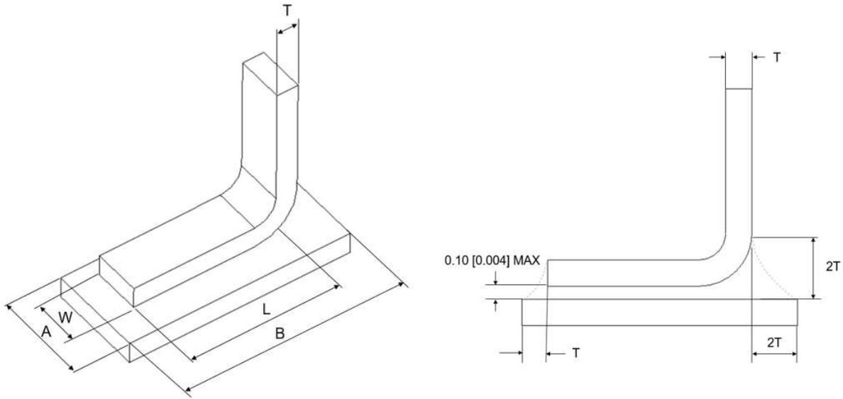
T = Thickness of solder tine
