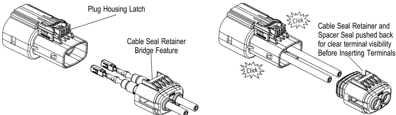
12. The spacer seal must be fully inserted until it stops inside the back of the plug housing as shown.
