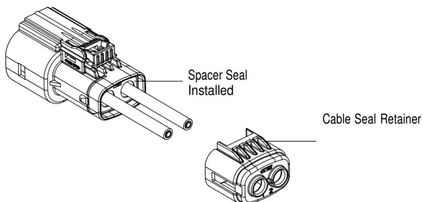
13. The cable seal retainer must be installed over the back of the plug housing so that the bridge feature is aligned with the plug housing latch. Both locking features must be fully engaged.
