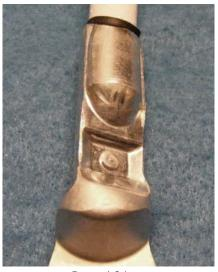
Rotated Crimp Terminal or splice rotated during crimping and locating shoulder was not aligned with scribe mark on die assembly nest.
