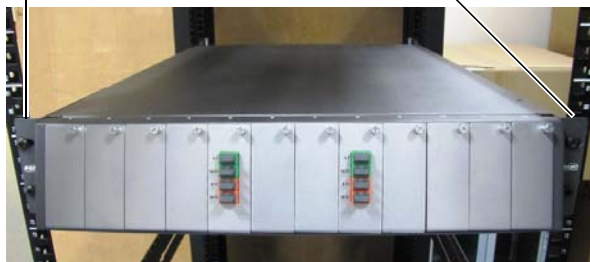
Front Brackets of Enclosure Secured to Rack (Ref)
