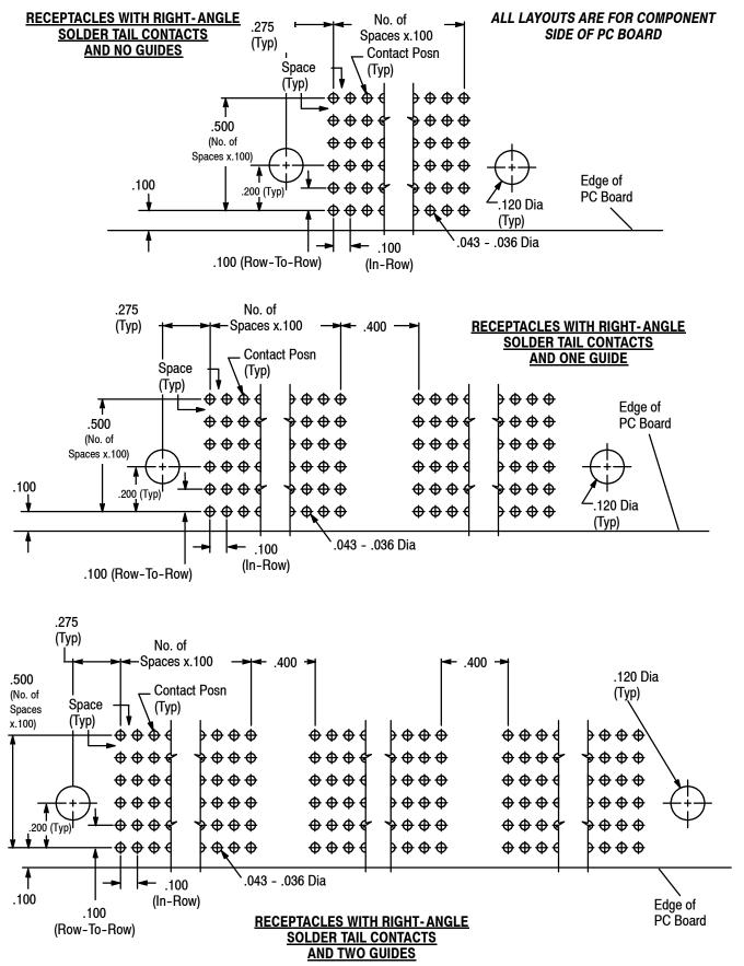
Figure 5 Receptacles with Solder Tails
