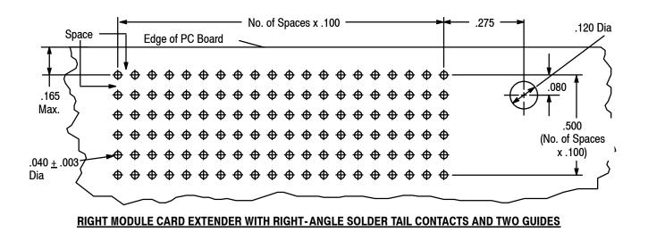
Figure 4 Headers with Right-Angle Solder Tails for Card Extender Applications
