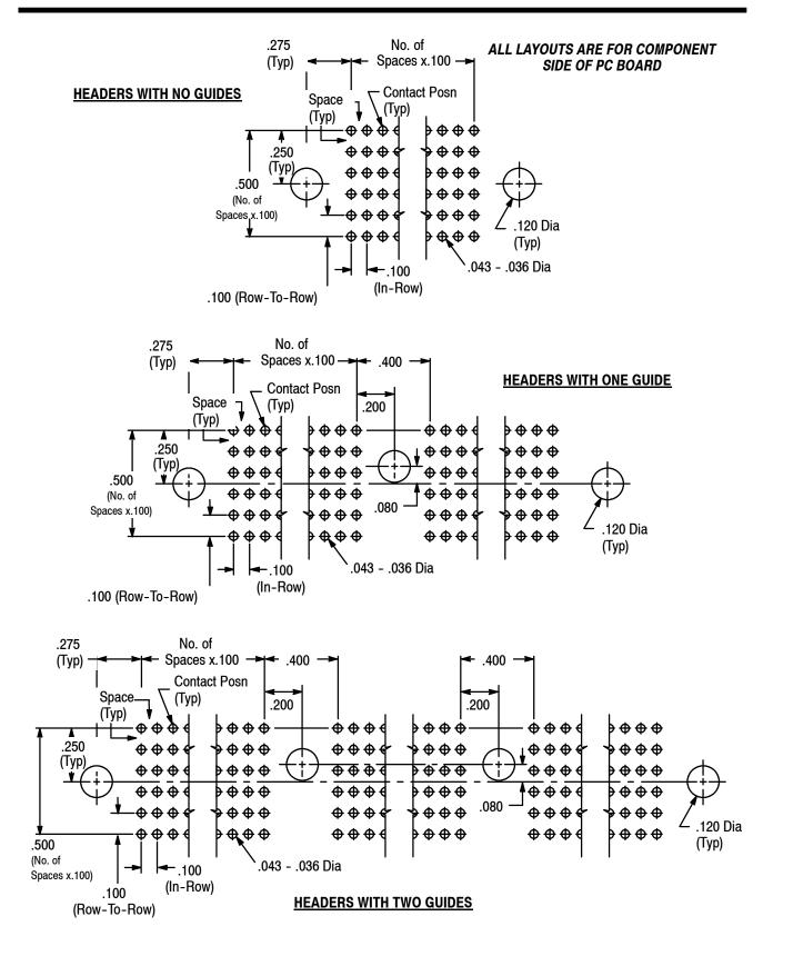
Figure 2 Headers with Straight Solder Tails
