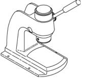
Manual Arbor Frame Assembly Without Tooling 58024-1 (Without Upper and Lower Tooling) (408-6923)
