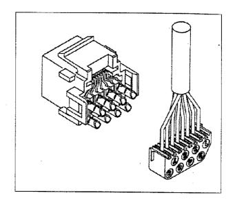
Terminate wires by pressing the Stuffer Cap over the Barrel Contacts.
