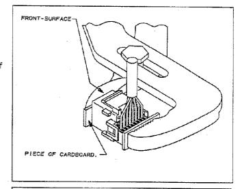
Inspect Jack assembly to ensure that Stuffer Cap is fully seated and that latches are locked at both sides.
