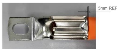
Figure 7: Crimp the ring tongue
