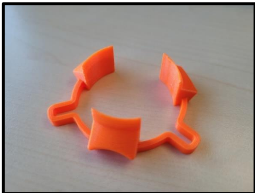
Figure 29: Auxiliary Tool #1 (3D-printed part) Auxiliary Tool to lift the clips of the cable cover
