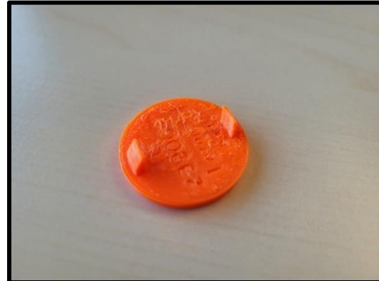
Figure 30: Auxiliary Tool #2 (3D-printed part) Auxiliary Tool to lift the hooks of the terminal fixation
