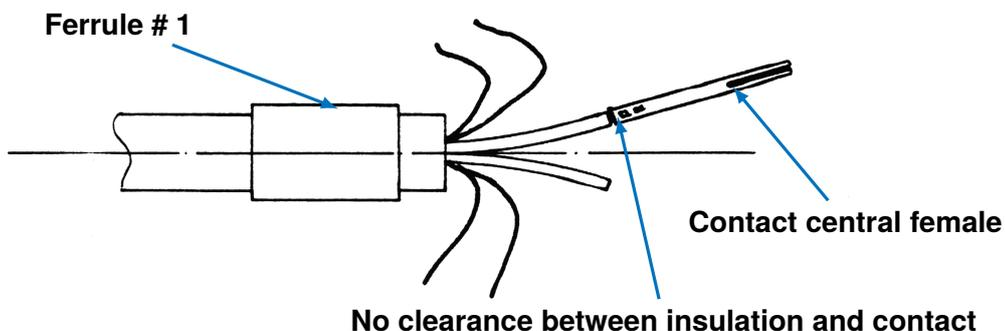
Figure 6: Female contact ready to be crimped
