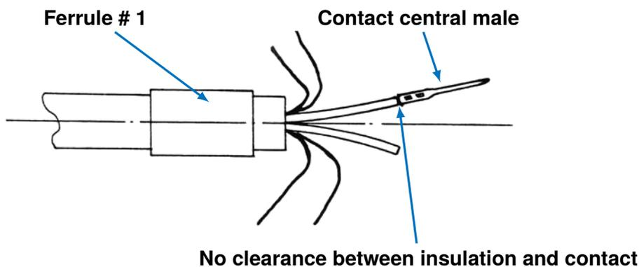
Figure 5: Male contact ready to be crimped
