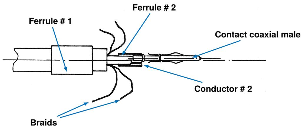
Figure 10: Assembly in position for crimping
