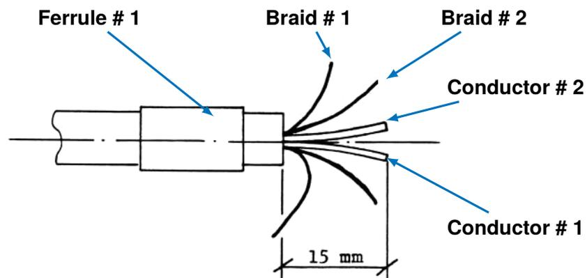
Figure 3: Cable preparation (step 2) Fillers removed
