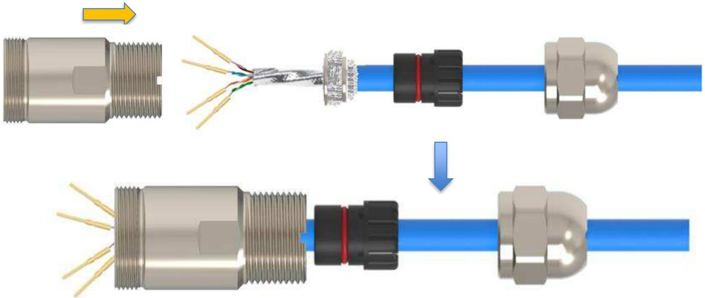
**9.7. Assemble the pressing screw with the metal body**
