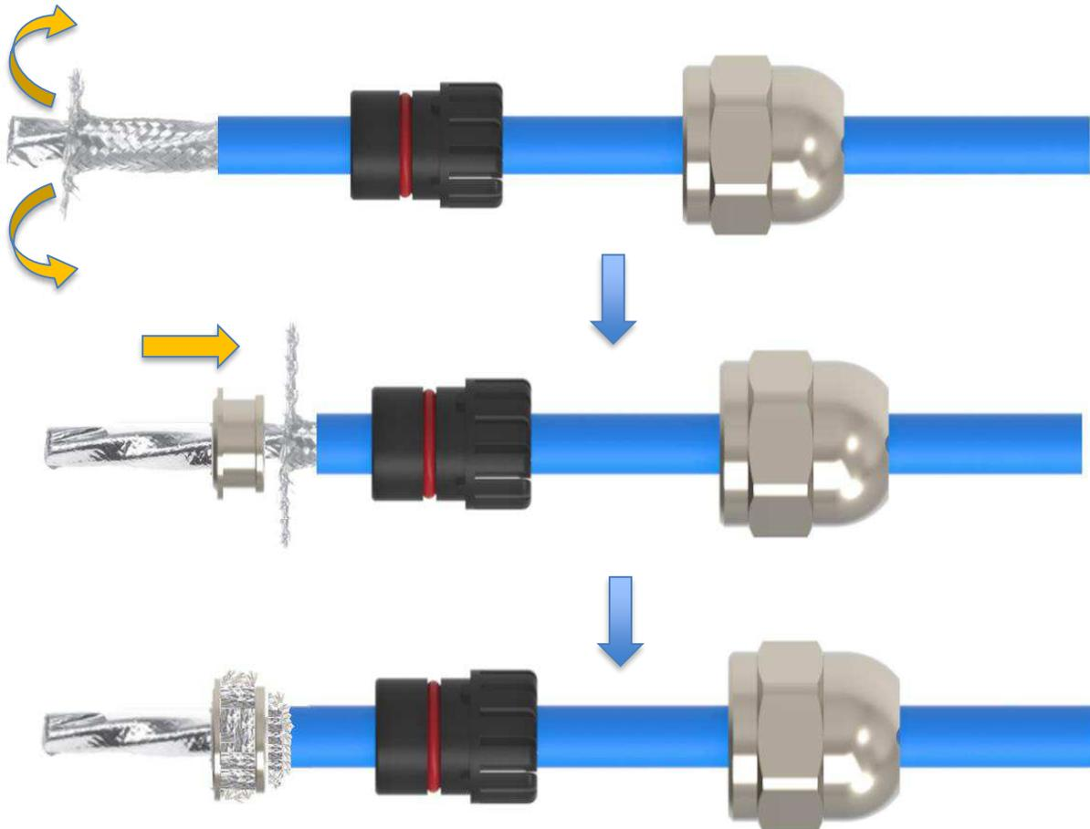
**9.4. Cut the foil as mentioned length only to ensure the wire twisting in the cable**
