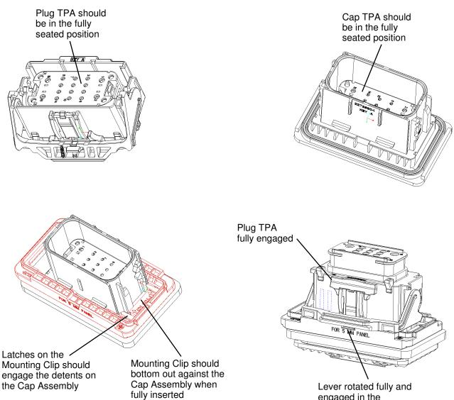
engaged in the Mounting Clip slot
