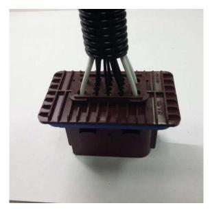
Figure 13 Slide the corrugate tubing onto the wires
