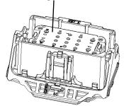
Using your fingers, squeeze the latches inward and pull the TPA out
