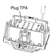
With the tool hooked onto the TPA latch, squeeze the latch inwards and pull on the tool. Repeat the process on the opposite side
