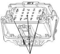
Press down on the ends of the plug TPA to move it to the fully seated position and the center to ensure a fully seated TPA
