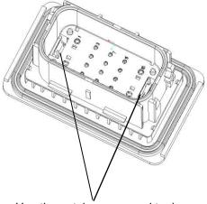
Use the notch on removal tool 776441-1 to press the latches inward and simultaneously press down to move the TPA to the fully seated position. Press on the latches one side at a time
