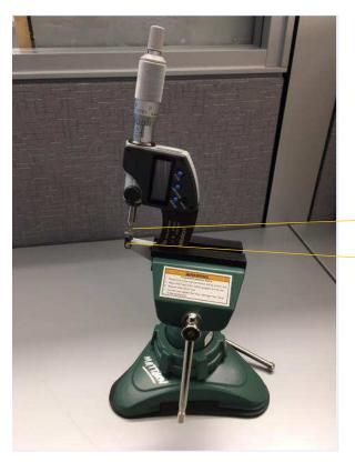
Measurement Tool Anvil Assembly (P/N 2844999-1)
