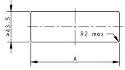
PLANE CUT OUT FOR BULKHEAD MOUNTING, THICKNESS OF WALL 1.3~3.0mm
