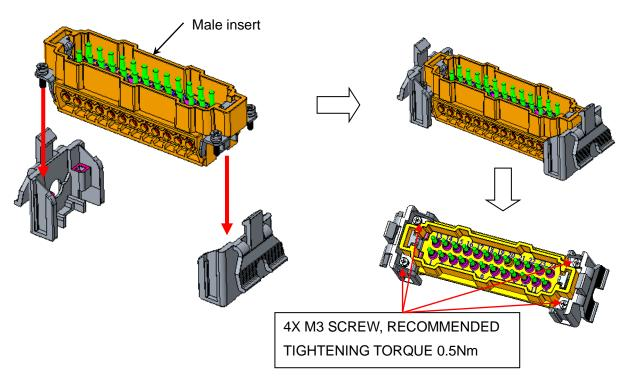
Step2. Assembly cables into Male insert.
