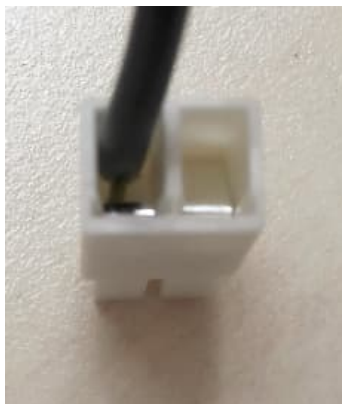
Visual Checking station-The wire should be bottom inserted
