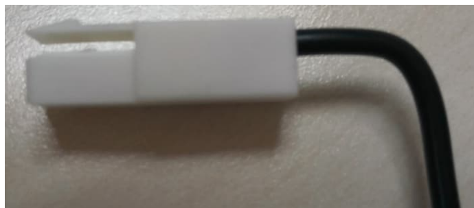
Visual Checking station-The wire should be bottom inserted
