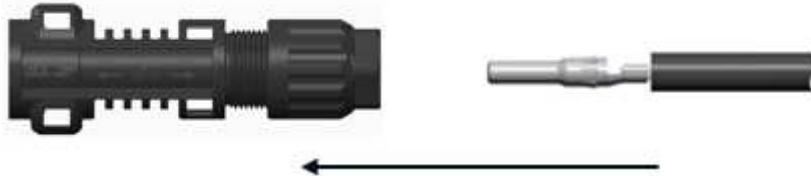
Figure 8 assembly: Insertion of contact with crimped wire lead of cable
