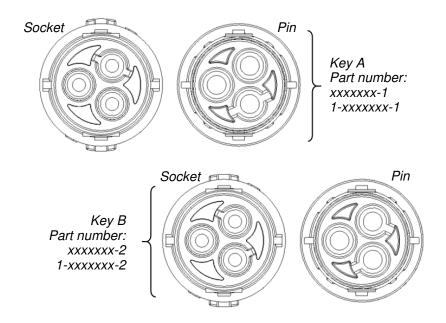
Figure 4, Polarization keys
