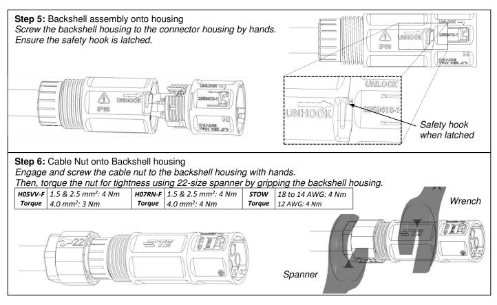
Figure 7, In-Line connector preparation
