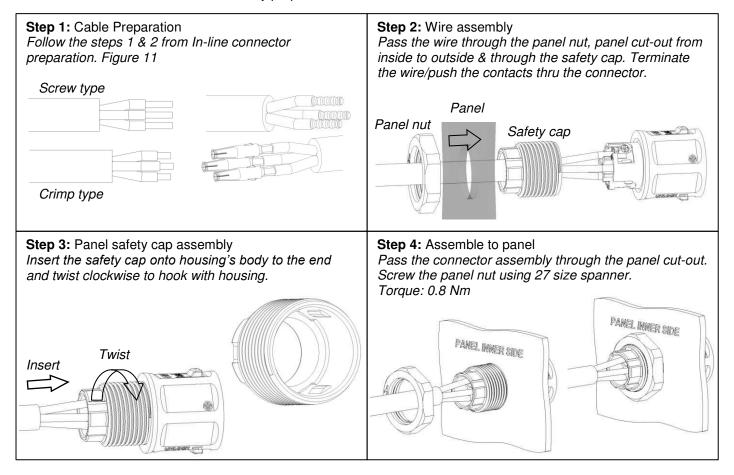
Figure 8, Panel Mount connector preparation
