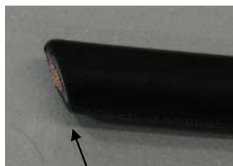
Jacket End max "10 °" cut, can be used
