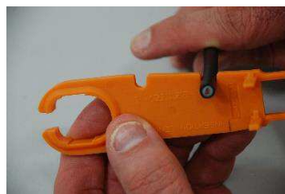
Figure 4.3 – determine if cable-outer-diameter is within min. and max. range with delatching-tool PN 2342988-1. Use the min. and max. cable openings on the tool to check if your cable is within the range yes or no.
