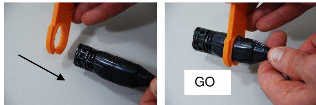
Figure 5.4 – Control termination with TE delatching-tool PN 2342988-1 (figure 7.1)
