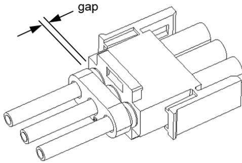
The wire seal should be inserted full depth into the housing wire receptacles (reference para. 5.0, assembly step 4, and Figure 3).
