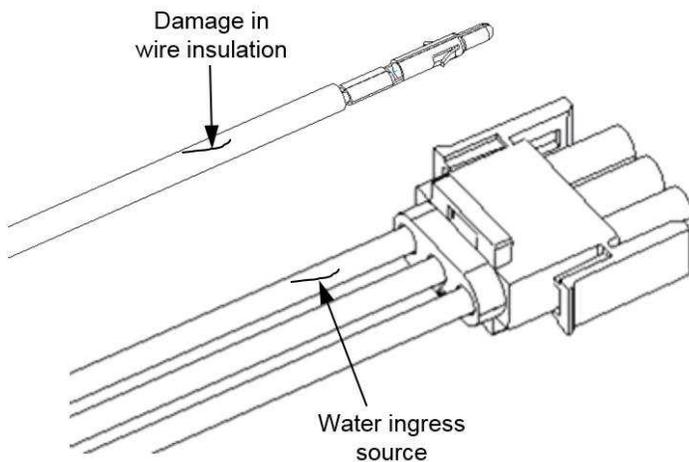
Wires should be carefully examined for damage prior to final installation into housings. Damage to wires insulation may provide water ingress path along inside of wire insulation and into the assembled connector.
