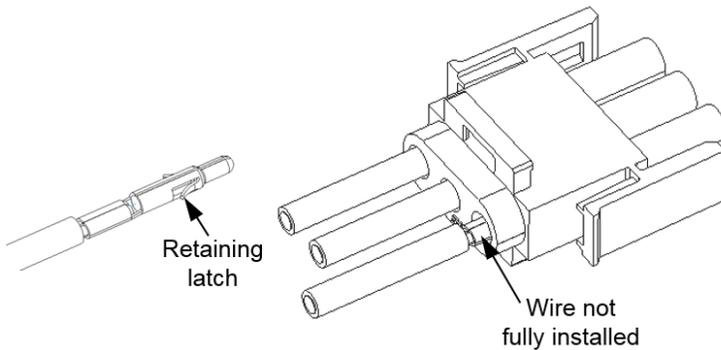
Crimped contacts should be fully inserted through the wire seal and into the housing so that contact retaining latches engage corresponding latch features inside the housing (reference para. 5.0, assembly step 9, and Figure 3, also ref. 114-1010).
