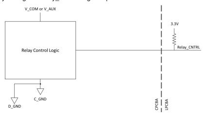
Figure 5. Relay Switching without Energy Metering (Example)
