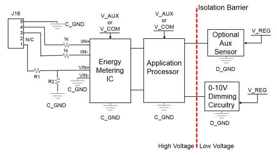
Figure 7. Energy Metering Implementation Architecture
