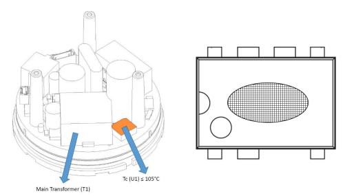
Figure 10 - Tc (U1) Location and suggested thermocouple placement
