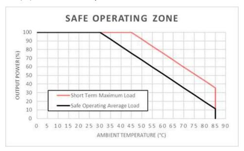
Figure 11 - Typical Application Derating Curve
