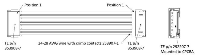
Figure 12. LCC Cable Assembly, TE p/n 2318043-1
