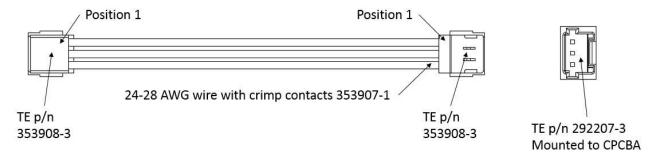
Figure 13. MPC Cable Assembly, TE p/n 2318043-2
