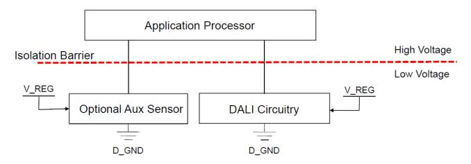
Figure 9. DALI Implementation Architecture on CPCBA
