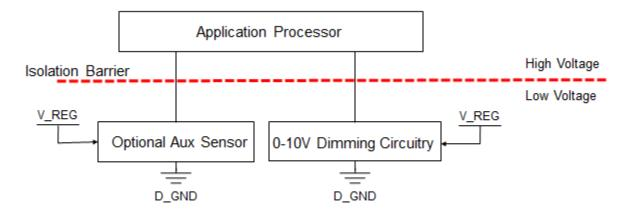
Figure 8. 0-10V Implementation Architecture on PCBA
