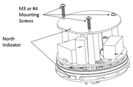
Figure 15. CPCBA Mounting
