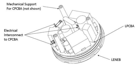
Figure 1. Control Node Layout using the LENEB
