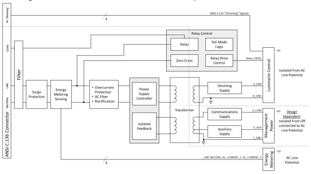
Figure 4. Detailed Block Diagram of LENEB
