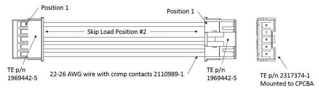
Figure 14. EMC Cable Assembly, TE p/n 2318044-1
