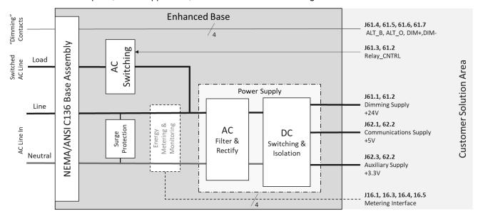
Figure 2. LENEB Functional Block Diagram
