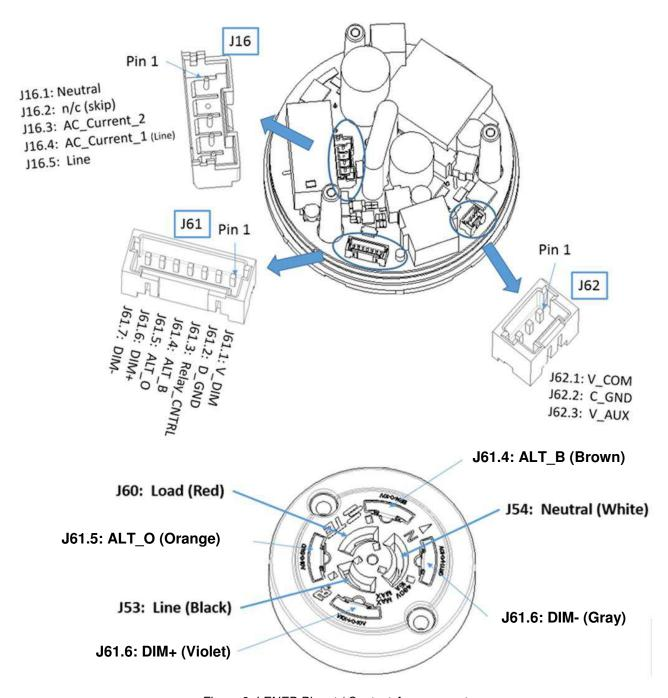
Figure 3. LENEB Pinout / Contact Arrangement
