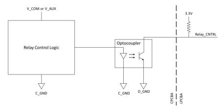
Figure 6. Relay Switching with Energy Metering (example)
