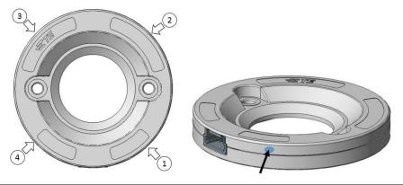
Step 2: Making hole in Top cover for Thermocouple wire
