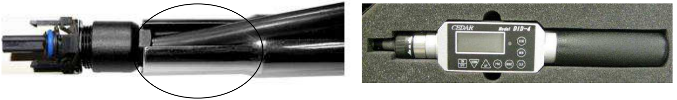
Figure 9 Tightening of the cable screw lock (Initial tightening torque is 1.0^{+0,2} Nm)
