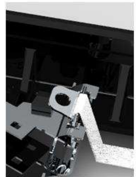
Remove the screwdriver to make S-clamp hold foil with contact rail
