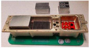
(2) Install Seating Tool into Receptacle Assembly
