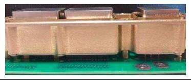
(3) Apply Insertion Force to Seating Tool to Install Connector to PC Board
