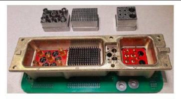
(1) Align EON Contacts/ Receptacle Assembly to PC Board
