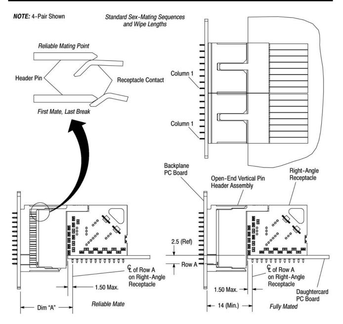
**NOTE:** The first mate, last break sequencing point is the first and last instance in a mating cycle where the pin comes in contact with the beam, but has not deflected the beam. The reliable mating point is the first and last instance in a mating cycle where the pin has completely deflected the beam, and the beam is supplying full normal force to the pin.
