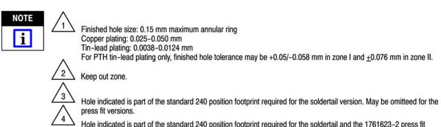
Hole indicated is part of the standard 240 position footprint required for the soldertail and the 1761623-2 press fit version. May be omitted for the 1761623-1 press fit version.
