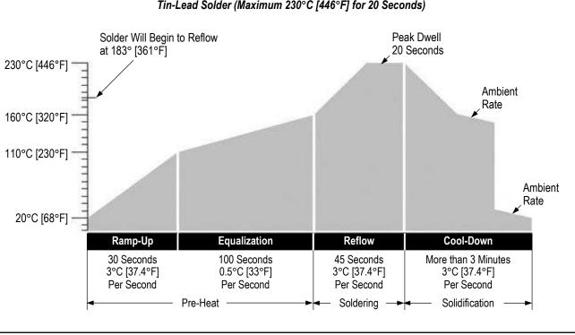
Reflow Soldering Process Cycle Tin-Lead Solder (Maximum 230°C [446°F] for 20 Seconds)
