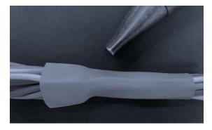
d. Ensure that the end of the heat gun does not touch the exterior of the tubing otherwise splitting may occur. Considering the temperature profile of hot air from the heat gun, maintain appropriate distance between hot gun and the tubing.
