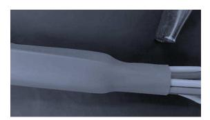
c. Work progressively to the end of the tubing ensuring uniform heat application. This can be achieved by either rotating the assembly or the heat gun. See figure 2. Ensure there is no air entrapment inside. *Minimum full recovery temperature: 340°C [644°F]*
